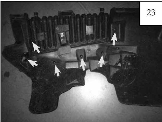
Plastic Phillips Head Tuf-Lok locations.
