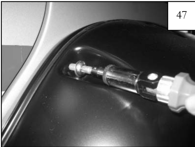
Start Screws/Washers through pocket holes in Outer Flare and into Threaded Clips installed in Step 18 (8 places). Do not tighten.
