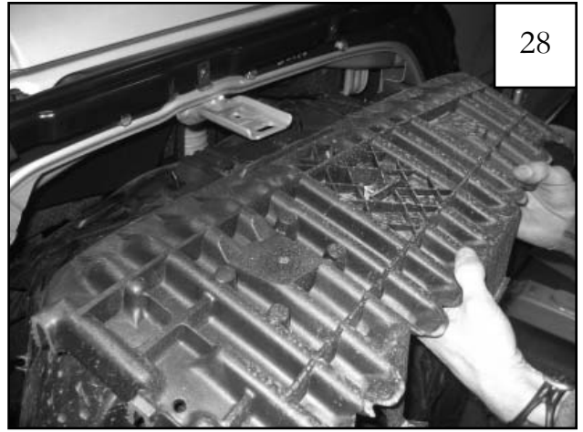
Replace factory inner structure/splash shield in fender as shown, sliding hole in structure over metal fender bracket.
