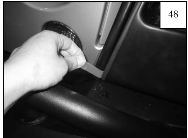
Pull tape liner from tape and press part to vehicle to secure adhesive backing. Tighten all Truss Head Screws first, then tighten all Torx Screws, moving from back to front.
